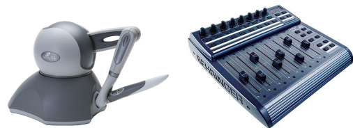
Figure 12: Left) The Omni haptic device from SensAble uses a mechanically tracked stylus that provides 6 degrees of freedom input (3D position + 3D orientation) and force feedback in 3 dimensions. Right) The Behringer BCF2000 is a fader controller device, with eight motorized faders that can be mechanically controlled from a computer application using the MIDI protocol.
