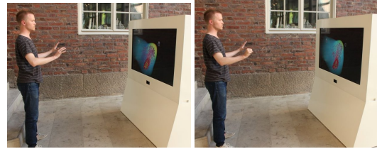
Figure 9: The user "grasps the heart" to rotate it with the right hand.
