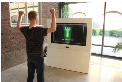
Figure 8: For skeleton tracking of the user, a one-time calibration pose is required initially.
