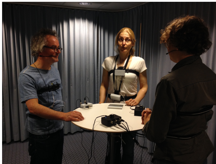
Figure 3: Recording setup. The white boxes are earlier prototypes of the RespTrack processors.
