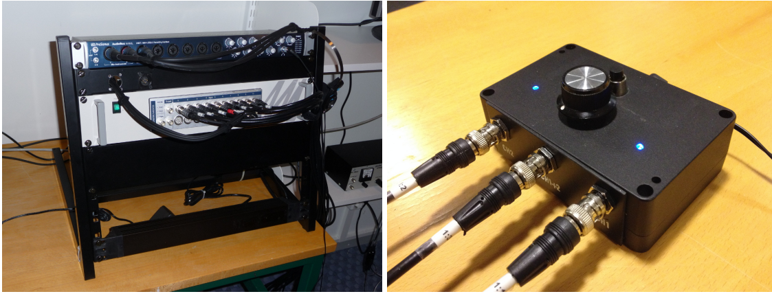
Figure 1: Data acquisition system: PowerLab alongside an audio interface (left) and a RespTrack belt processor (right).
