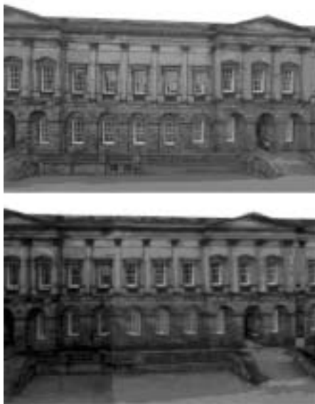
Figure 3: A frame blended using frequency-dependent blending at the top, and linear blending on the bottom. Looking at the perspective at the two ends of the building it is evident they are derived from different source photographs. The geometric proxy for this façade is just a plane.
