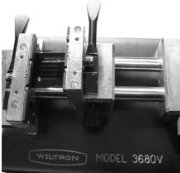
Fig.7 Filter mounted in standard Wiltron test fixture.
