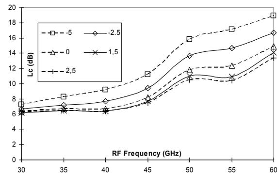
Fig 3 Down conversion loss of the pHEMT mixer with LO-power as parameter
