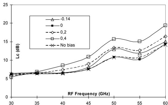
Fig 5 Down conversion loss of the pHEMT mixer with LO power of 2dBm and  $V_{DS}$  as parameter
