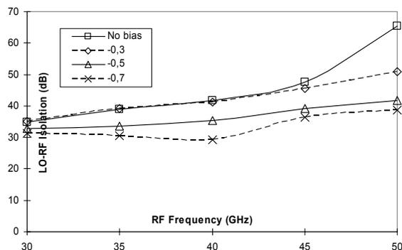
Fig 6 LO-RF isolation for the pHEMT mixer with LO power of 2dBm and  $V_{GS}$  as parameter
