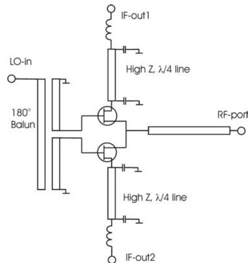
Fig 1 Schematic of the mixer
