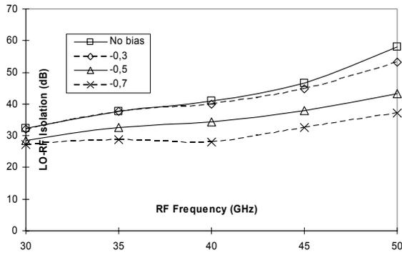
Fig 7 LO-RF isolation for the mHEMT mixer with LO power of 2dBm and  $V_{GS}$  as parameter
