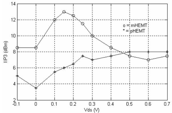
Fig 11 IIP3 with LO power of -4 dBm and  $V_{DS}$  as parameter
