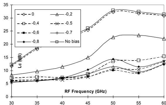
Fig 4 Down conversion loss of the pHEMT mixer with LO power of 2dBm and  $V_{GS}$  as parameter
