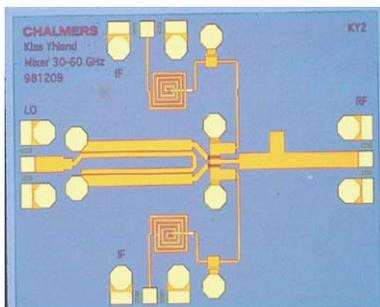
Fig 2 Photo of the MMIC balanced mixer. The design was made by Klas Yhland at MC2.
