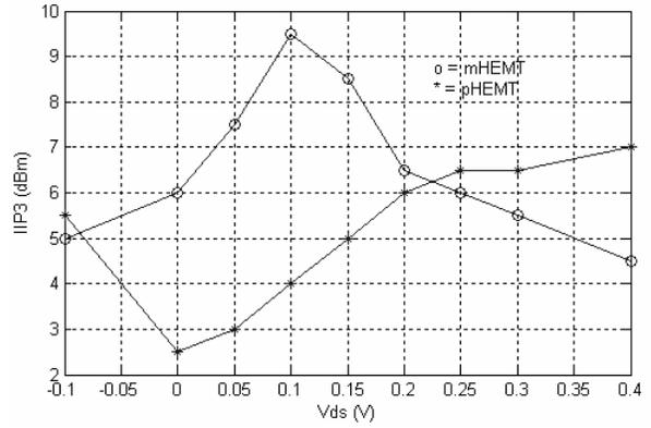
Fig 10 IIP3 with LO power of -8 dBm and  $V_{DS}$  as parameter
