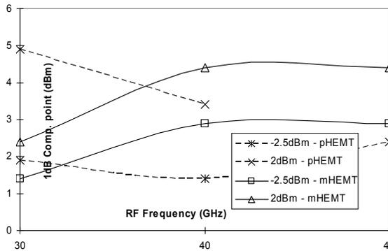
Fig 8 1 dB compression point for both the pHEMT and mHEMT mixer with LO-power as parameter
