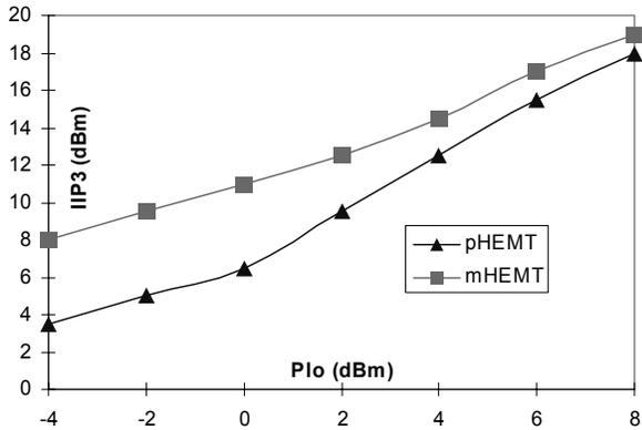
Fig 9 IIP3 with LO-power as parameter and no  $V_{DS}$  bias applied
