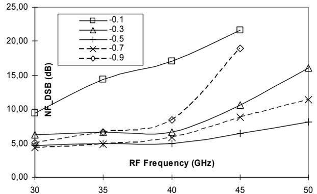
Fig 12 Down conversion  $NF_{DSB}$  of the pHEMT mixer with LO power of 2dBm and  $V_{GS}$  as parameter
