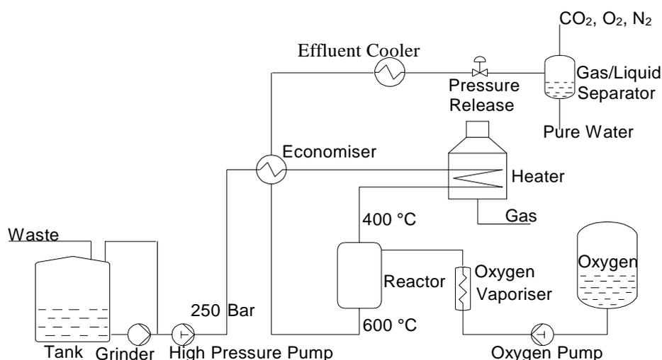
**Figure 4** Simplified flow schema of the pilot plant
