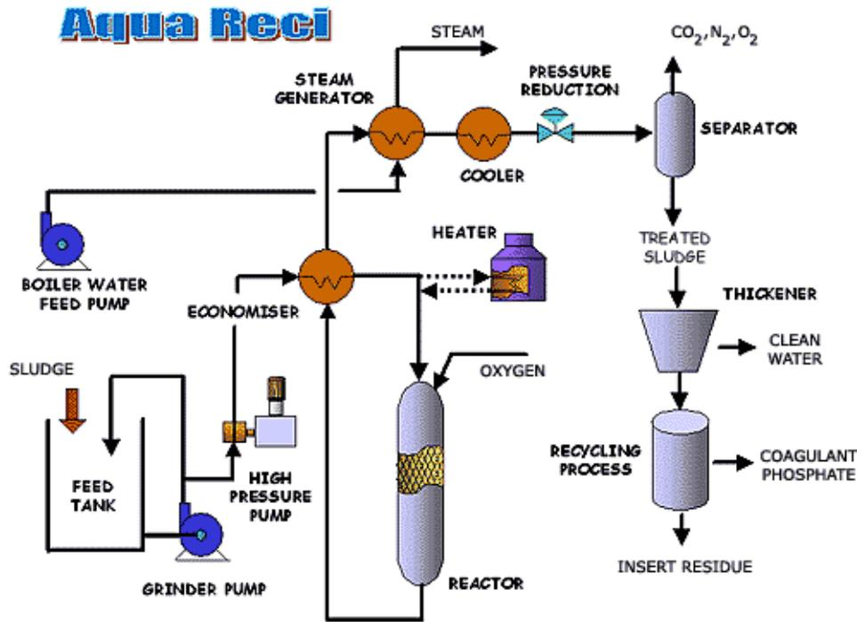
**Figure 6** Simplified flow scheme of the Aqua Reci™ process
