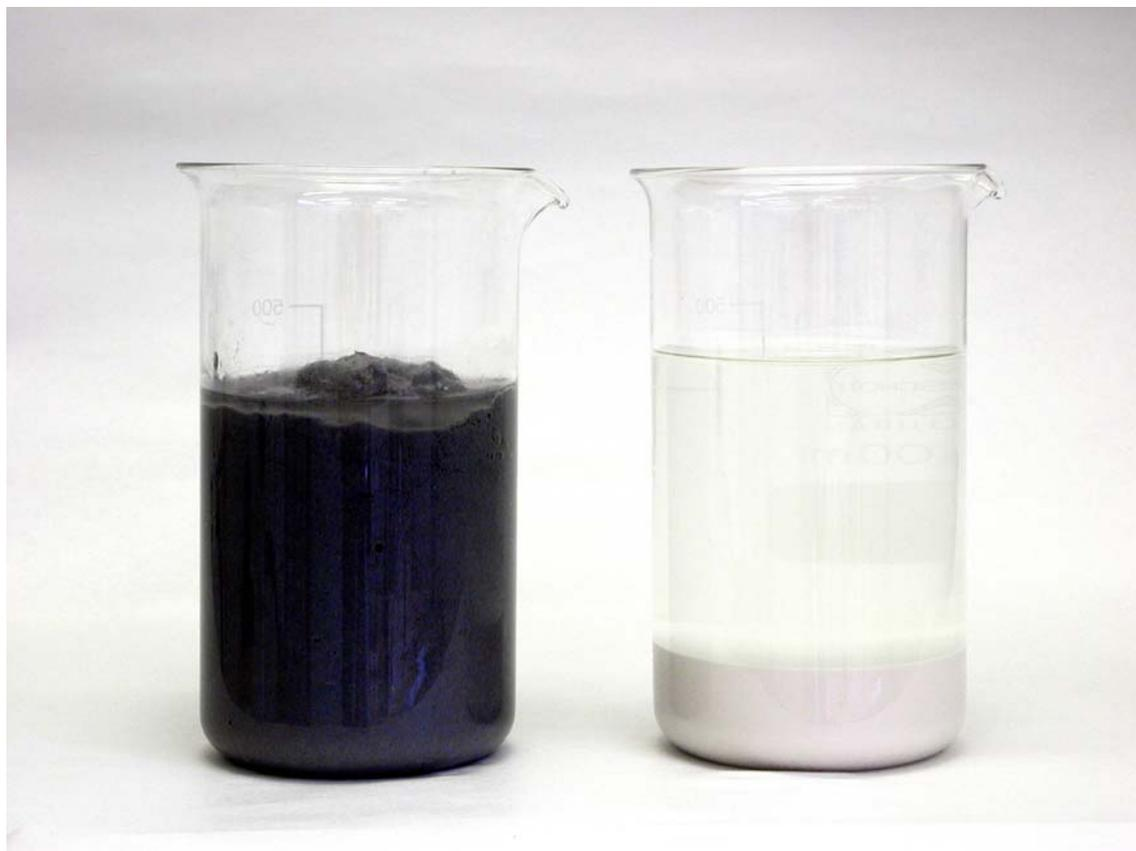
**Figure 5** Feed de-inking sludge and effluent after SCWO treatment
