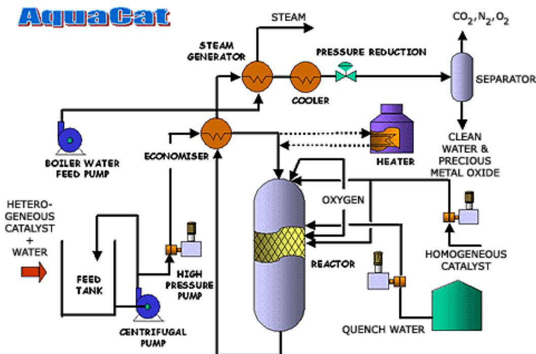
**Figure 8** Flow scheme of the AquaCat<sup>®</sup> process
