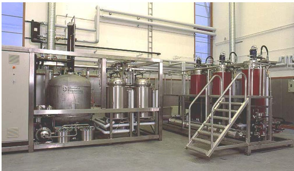
**Figure 3** Xtractor™ 500/1000, 1000 kg/h, 500 bar scCO<sub>2</sub> extraction plant
