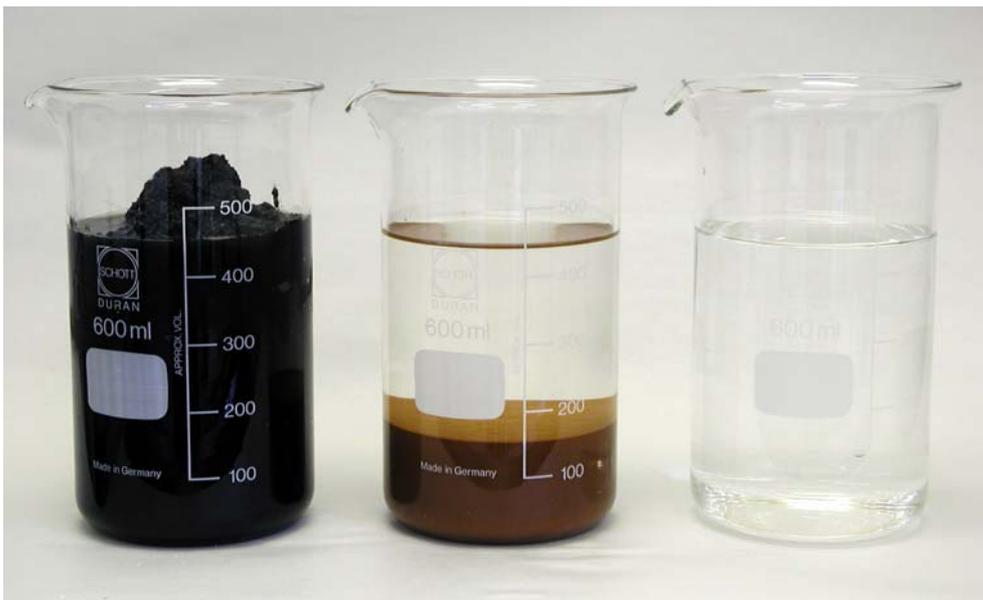
**Figure 7** Feed sewage sludge, effluent from SCWO process and decanted water phase
