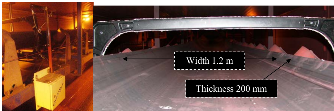
Figure 4. The figure to the left shows the conveyor belt with the mounted reader device. The figure to the right shows the antenna of the reader and the dimensions of the conveyor belt.
