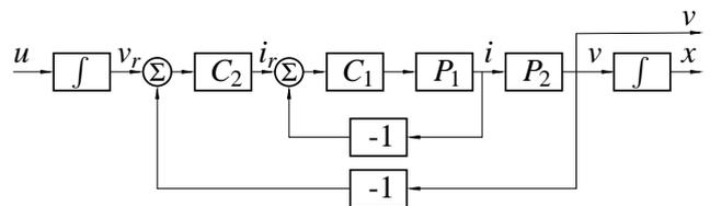
Figure 4: Cascaded control structure for the cart control.
