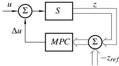
Figure 14: A schematic view of how the MPC-feedback is introduced.
