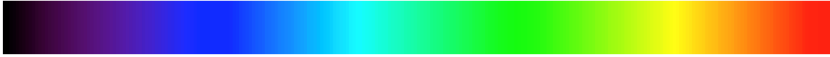
Figure 3. The “rainbow” palette is a common color scheme used for coding numeric values as colors in data visualization. Unfortunately this palette is difficult or impossible for the human visual system to interpret properly. Some color transitions (blue to green and yellow to red, for example) occur very quickly, which introduces false contrast, while other colors (green in particular) cover wide ranges of the palette, obscuring detail. (Image courtesy Robert Simmon, Sigma Space/NASA Goddard Space Flight Center.)
