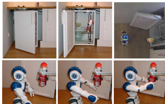
Figure 6: Fridge door opening( upper left ), fridge gripper bringing the can out( upper middle ), tracked image from the camera ( upper right ), Pre-defined robot arm movements after reaching the desired position for grasping the object( bottom left, bottom middle and bottom right )
