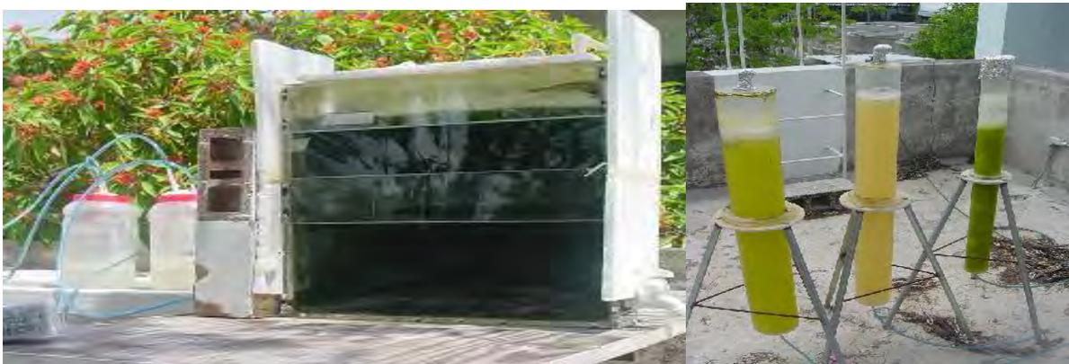
Fig 1. Pictures showing two different types of solar photobioreactors for the production of microalgal biomass at external conditions: flat panel reactor and vertical tube reactors.
