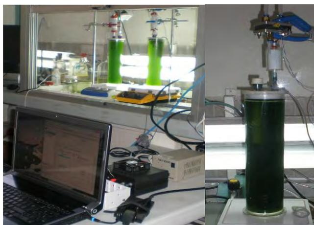
Fig. 2. Pictures showing the reactors for biohydrogen production with microalgae under laboratory conditions.
