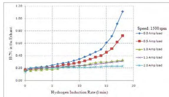
Fig. 10 Effect of hydrogen induction rate on  $\text{HC}$  emission at difference loading
