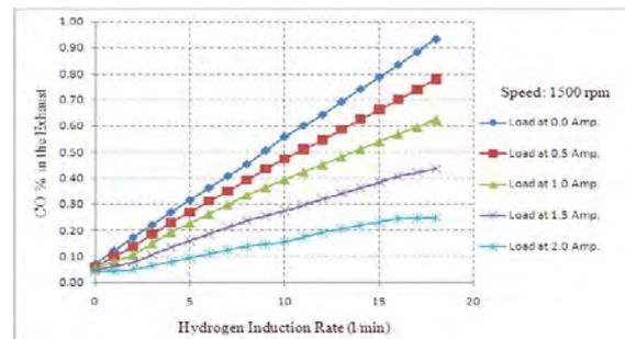
Fig. 8 Effect of hydrogen induction rate on CO emission at difference loading
