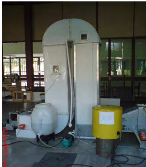
Figure 2. The LDAC packed-bed dehumidification unit as viewed from the MERC Energy Laboratory.
