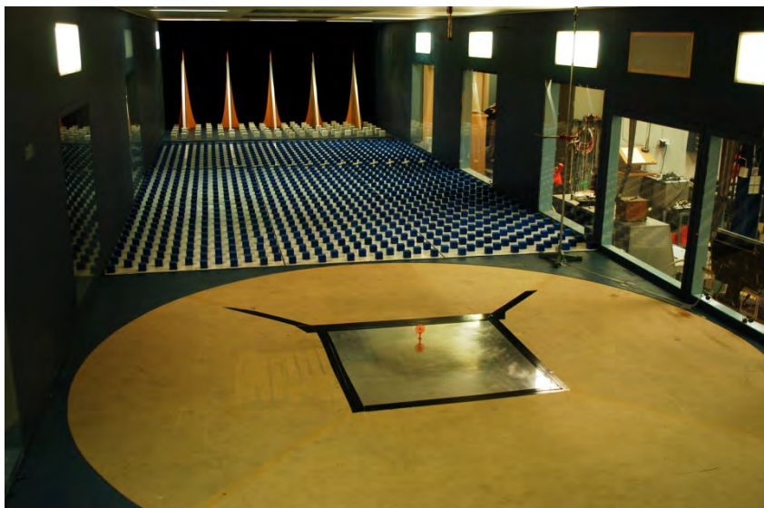
Fig. 4 Wind tunnel with one wind turbine model placed on the pressure plate along line 10 in Fig.3
