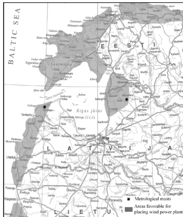
Fig. 1. The coastal map of Baltic countries with the places of interest for siting WPPs indicated.
