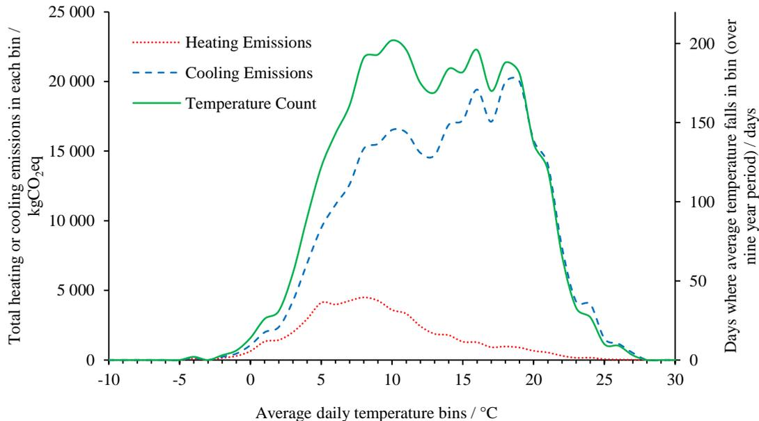
Fig. 2. Total CO<sub>2</sub>eq emissions from example building heating and cooling demands and temperature frequency of occurrence in daily average temperature bins of 1°C
