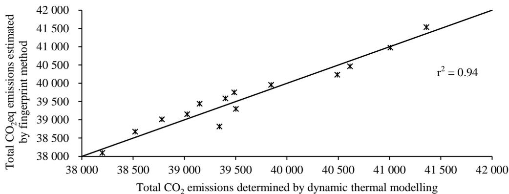
Fig. 4. Comparison of CO<sub>2</sub>eq emissions between estimated figures using fingerprint method and dynamic thermal simulation
