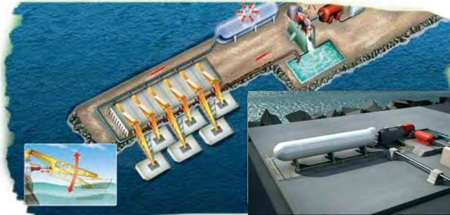
Figure 1: Wave power plant using high pressure system as described in Estefen et al [1]
