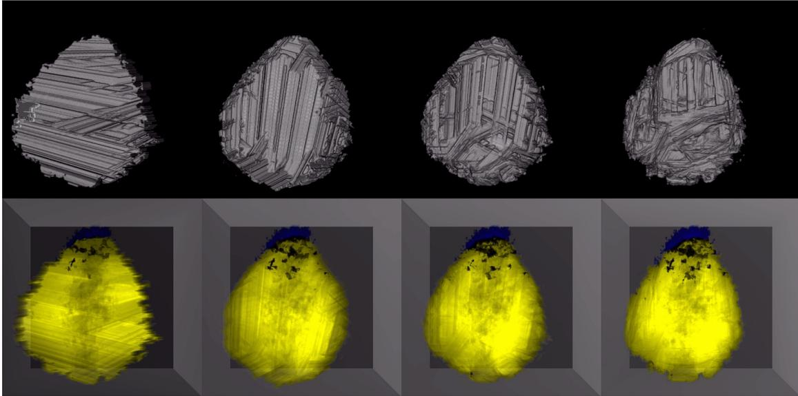
**Figure 5:** The upper row shows surface renderings of the the visual hull reconstructions for increasing numbers of silhouette images (from left to right: 3 images, 7 images, 14 images, and 35 images). The bottom row is a visualization of the subtraction volumes for increasing numbers of silhouette images. In all cases, reconstructions were applied for a volume segmented with a threshold of 0,01.
