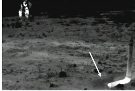
**Figure 1:** Infra-red (IR) image showing methane gas leaking from a deduction pipe.
