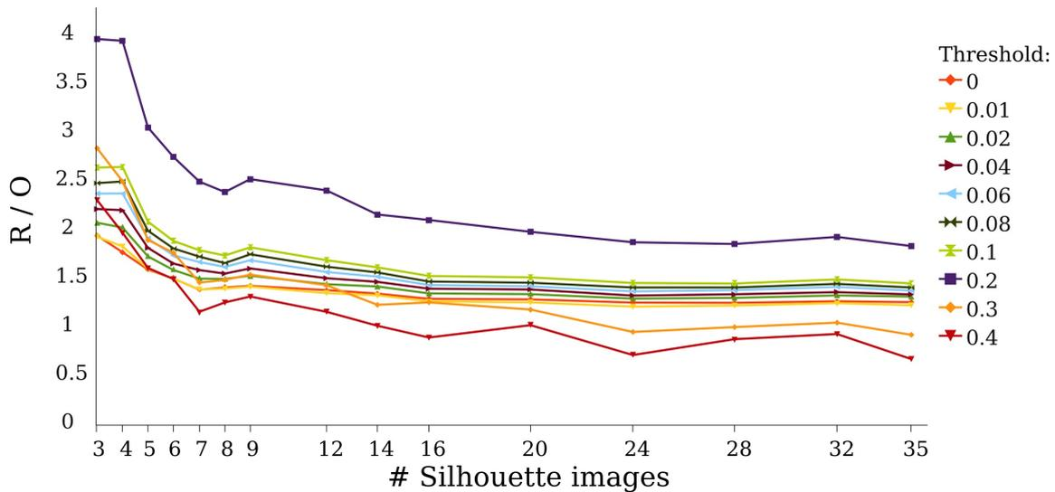
**Figure 6:** Diagram showing the ratio of the volume sizes  $R/O$  of the reconstructed volume and the original (reference) volume for increasing numbers of silhouette images. Data series are plotted for the same raw data volume but with varying segmentation thresholds.
