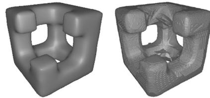
**Figure 2:** An example of a polygonal model (left) and its volumetric reconstruction using visual hull methods (right).
