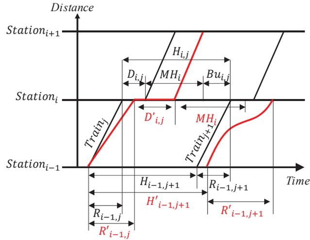
Figure 6: Mechanism of train delay propagation
