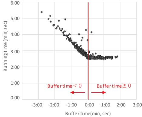
Figure 7: Relationship between Buffer time and Running time
