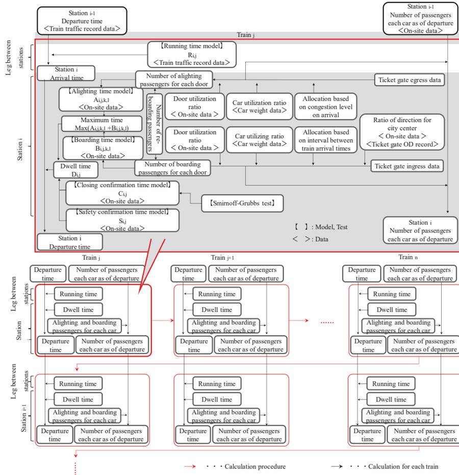
Figure 2: Simulation flow
