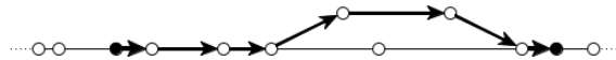
Figure 3: A route defined as a path in the graph, starting with an entry signal.
