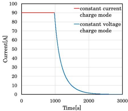
Fig.3 Current characteristic of charging to represent in (3)
