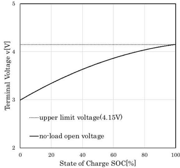
Fig.1 No-load open voltage of LIM-30H made by GS Yuasa Co. (per a cell)
