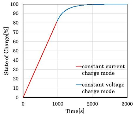
Fig.4 SOC characteristic of charging to represent in (4)
