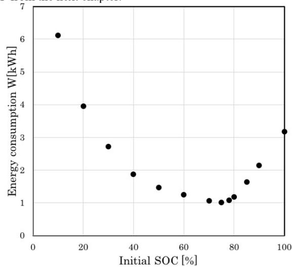
Fig.5 Relevance between Initial SOC and energy consumption
