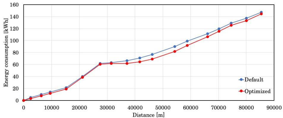
Fig.14 Transition of integrated value of the energy consumption of the default and the optimized timetable
