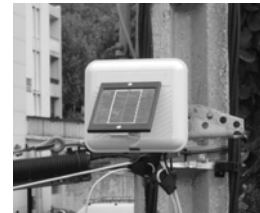
Figure 6: A solar powered gateway.
