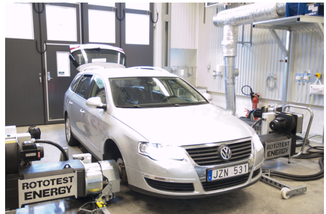
Figure 2. Vehicle mounted at Vehicular Systems chassis dynamometer laboratory at LiU.
