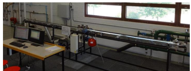
Figure 1. Educational heat exchanger system.
