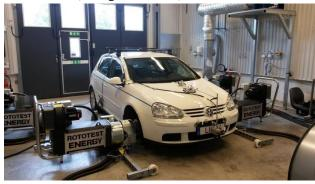
**Figure 1.** The Golf V used for measuring powertrain data connected to chassis dynamometers at the vehicle propulsion laboratory at Linköping University.
