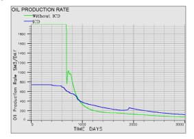
Figure 11. Trend of Oil Production Rate.
