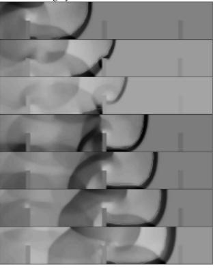
**Figure 5:** Simulated density gradients of shock-flame-obstacle interactions for the 40 mm channel with repeated obstacles. The images show the failure of detonation. Stoichiometric hydrogen-air at 293 K and 1 atm.
