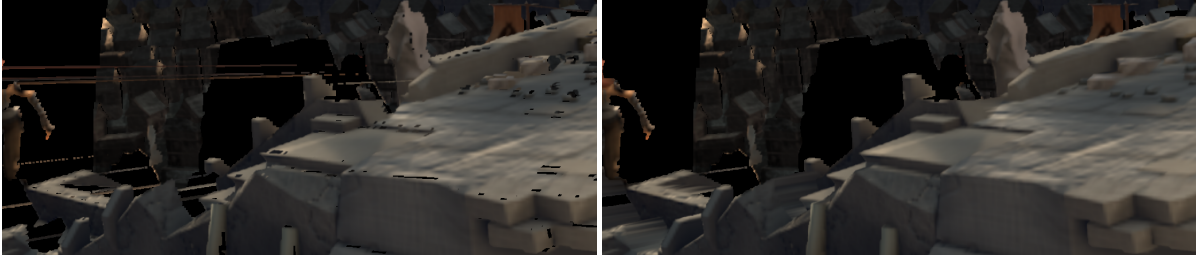
Figure 3: Wrongly connected mesh (left): connections over object boundaries (causes stripes) and missing connections (causes black spots). Our meshing algorithm was able to remove most of these artifacts (right). (detail from the temple2 sequence)
