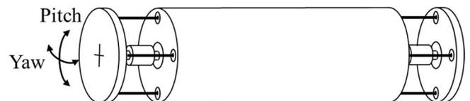
Figure 22. Actuation in pitch and yaw rotational direction at left and right end of the robot arm segment.
