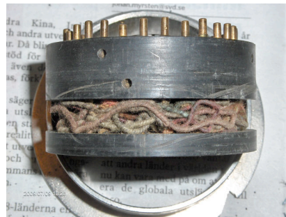
Photo 2: Opened rotor A133. Source: FRA
