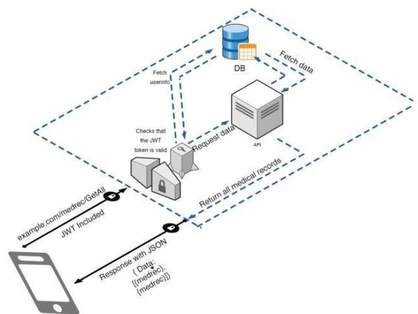
**Figure 7** Example of a request to the system.
