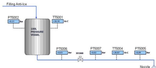
Figure 2. P&ID for the experimental test rig
